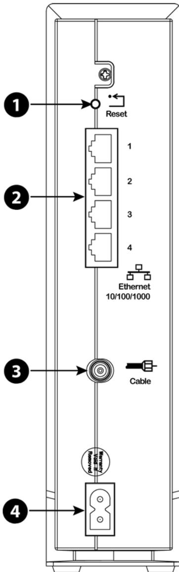
1. **Reset button:** resets the Data Gateway as if you power cycled the unit. Use a pointed non-metallic object to press this button.
