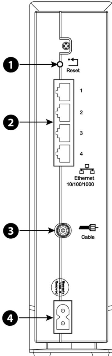
1. Connect one end of the coax cable to the cable outlet or splitter, and the other end to the Data Gateway's Cable connector (**3**). Tighten the connections by hand, then tighten an additional 1/8 turn with a wrench.
